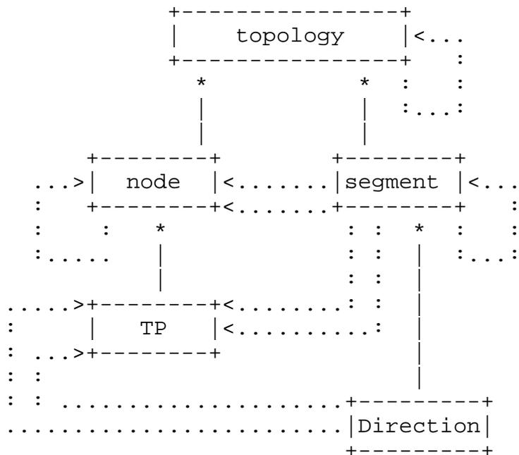
The basic information model works as follows: A service topology contains service nodes and segments. A segment connects two nodes (a source and a destination) and have direction, may be unidirectional or bidirectional. unidirectional is one where traffic is passed through a set of SF nodes in one forwarding direction only. Bidirectional is one where traffic is passed through a set of SF nodes in both
