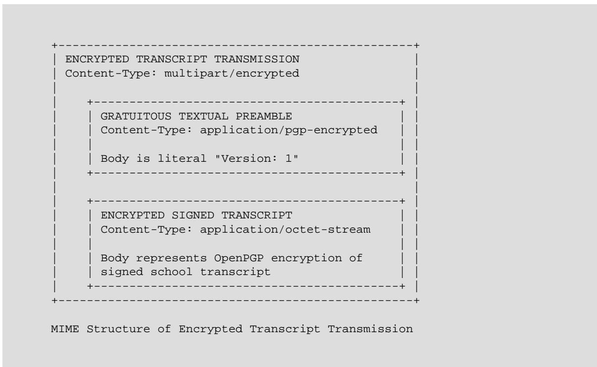
Figure 8: MIME Structure of Encrypted Transcript Transmission
