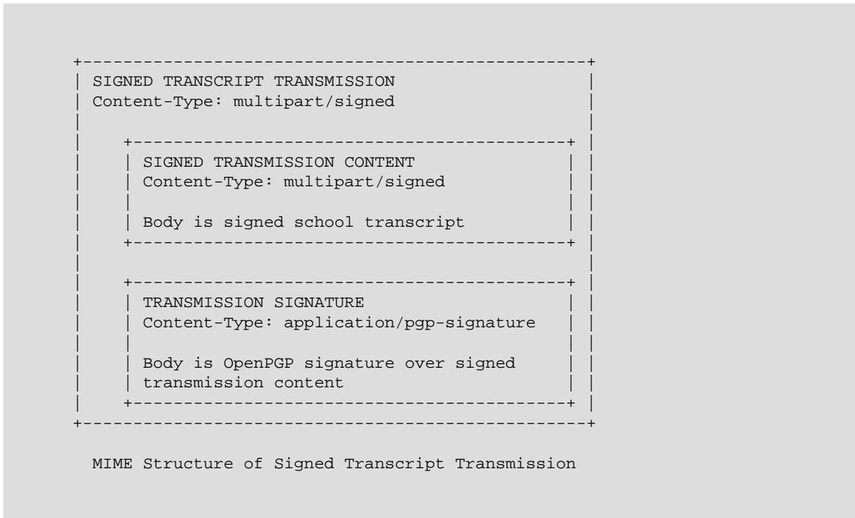
Figure 9: MIME Structure of Signed Transcript Transmission
