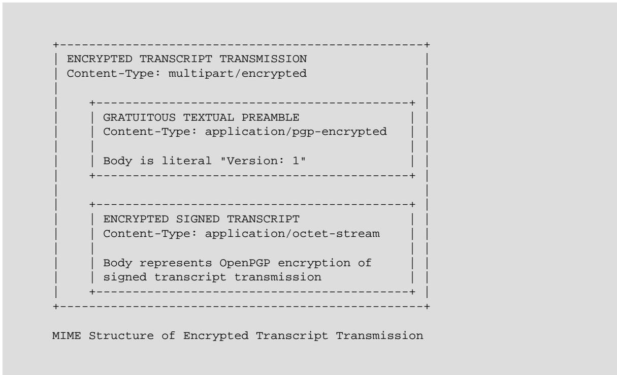
Figure 10: MIME Structure of Encrypted Transcript Transmission
